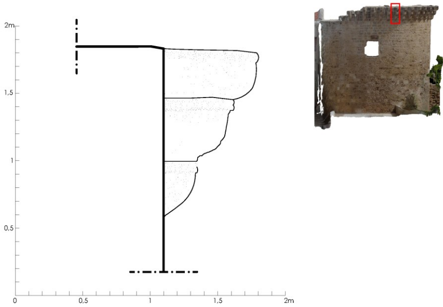
Fig. 10- Detail of the corbels, side elevation (Griffo, 2018)
