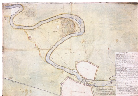
Fig. 3- Design for straightening of a tract of the Tanaro close to the city, signed by Clarici and drafted in 1593
