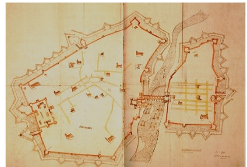
Fig. 6- Use of waterways for the defence of the urban environment in a planimetry study by Giovanni Pietro Pelucco, drafted in 1625
